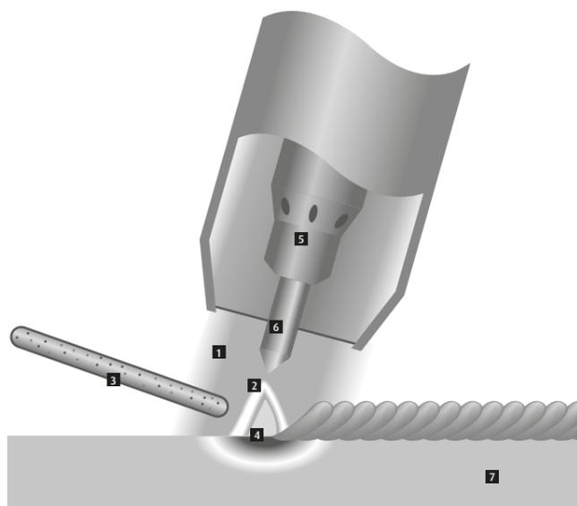
Schematic of the TIG welding process
