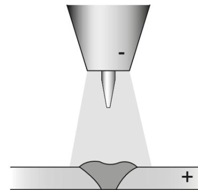
GTAW with DCEN produces deep penetration because it concentrates the heat in the joint area. No cleaning action occurs with this. The heat generated by the arc using this polarity occurs in the work thus a smaller electrode can be used as well as a smaller gas cup and gas flow. The more concentrated arc allows for faster travel speeds.
